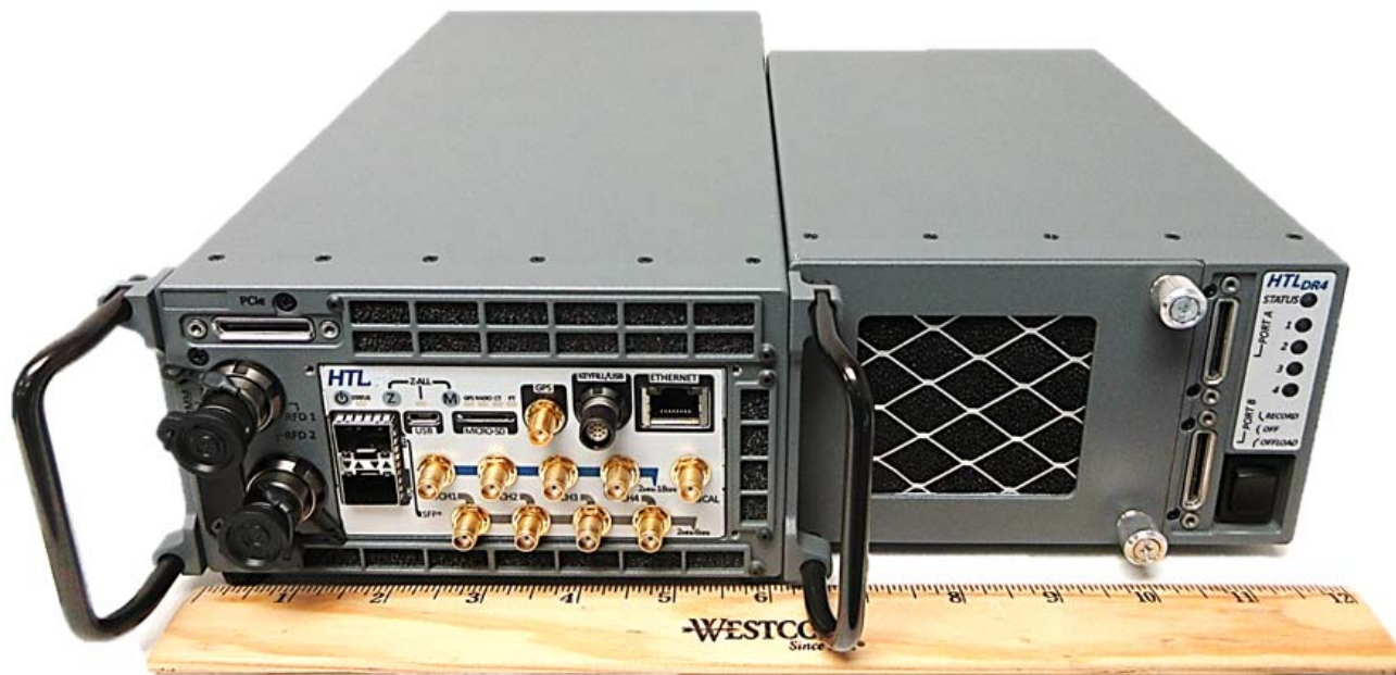
DR-4 Small Form-Factor Wideband Recorder (shown with HTLx-U)
